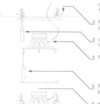
1 Cut out hole in ceiling or wall using template as cutting guide, or to a diameter of 198 - 202mm (7 1/2 in).
