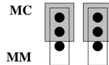
PHONO JUMPER SETTING FOR MOVING COIL (MC)
