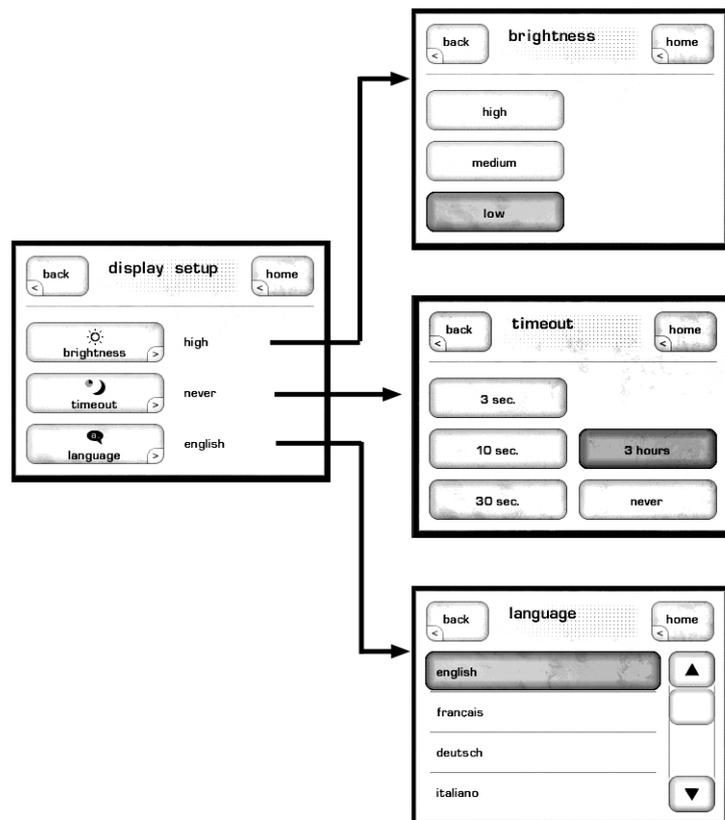
This button brings up the **display setup** menu. It allows you to configure the CP-500's LCD screen *brightness*, the display *timeout*, and the *language* used in the touchscreen and menu system.
