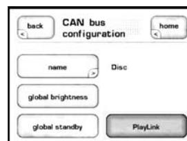
Once you have selected the input press **back**, then select **configuration**. PlayLink is activated and disabled through the PlayLink icon on the CAN-Bus configuration screen.
