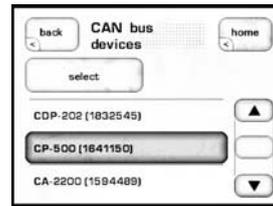
Highlighting a unit on the CAN-Bus devices screen identifies it as the **target unit**. The front panel LEDs of the target unit will start flashing (unless you highlight the unit that you are using to access CAN-Bus).
