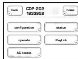
The first step in using PlayLink is to choose the **input** you wish to be selected when play is pressed on the disc player. Press the **PlayLink** icon, then select the correct input from the list.
