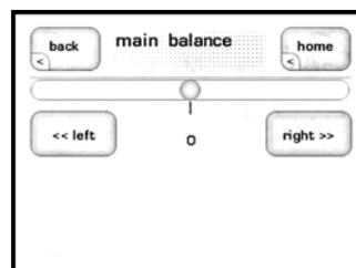
The **main balance** control gives you both a numeric and a graphical indication of the current balance setting for the CP-500.
