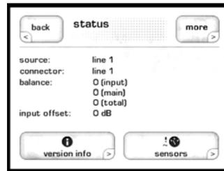
The **status** screen provides several items of information about the current operation status of the CP-500, as well as access to information on the software used in and the internal sensors of the CP-500.
