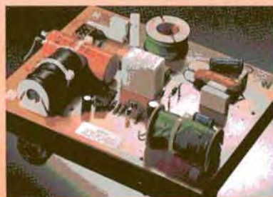
Sophisticated computer-optimized fourth-order Butterworth squared crossover network incorporates B&W's patented APOC system.
