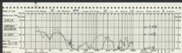
Harmonic Distortion for 10 volts input (solid curve = 2nd, dotted curve = 3rd.)
