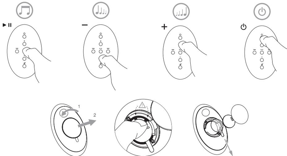
The MM-1 can be operated either from the controls on the sides of the powered speaker or from the remote control handset (illustration top). If the remote handset is to be used, its battery-insulating tab must first be removed. This is illustrated above.
