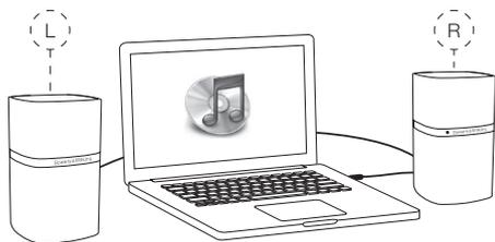
The two MM-1 speaker units are intended to be desk mounted, one either side of a computer monitor. The powered speaker should be on the right side of the monitor and the slave speaker on the left hand side. Do not position the speakers too far apart if your are sitting close to the monitor. The triangle formed by the two speakers and the listener's head should be approximately equilateral. The MM-1 speaker positioning is illustrated above.
